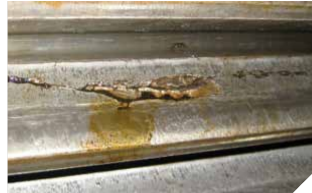
Visual inspection after cleaning uncovered a crack on a gear tooth
