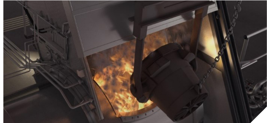
Excellent gas capturing during charging of matte
