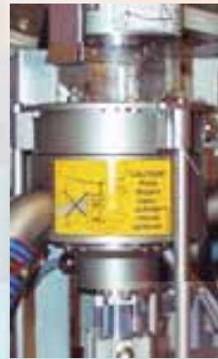
In the Freeness module an ultrasonic cleaner ensures that the measuring cell is clean for the next analysis.
