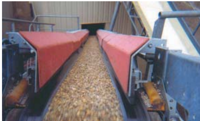
Guide and sealing chute over full length.
