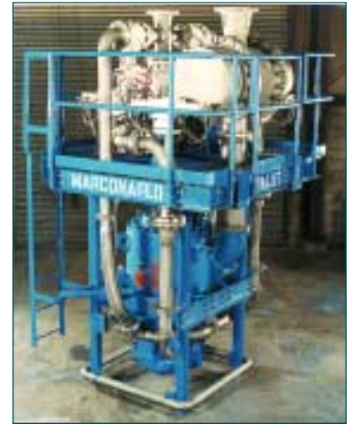
DYNAJET® SUBMERSIBLE With hydraulic power unit and density control system
