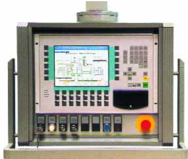
Multi-information terminal for process data visualization and online help
