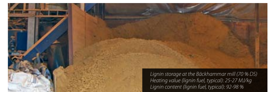
Nordic Paper - Bäckhammar, Sweden. Plant data: • 175 000 ton SW pulp • Kappa number 40 • BL solids about 70% • 690-700 ton DS/day • 6 000 - 10 000 ton lignin/year • Lignin DS: 70 %
