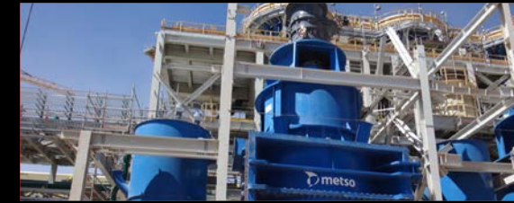
Vertimill® - stirred milling technology
