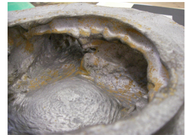
Figure 7 - Usure et corrosion
