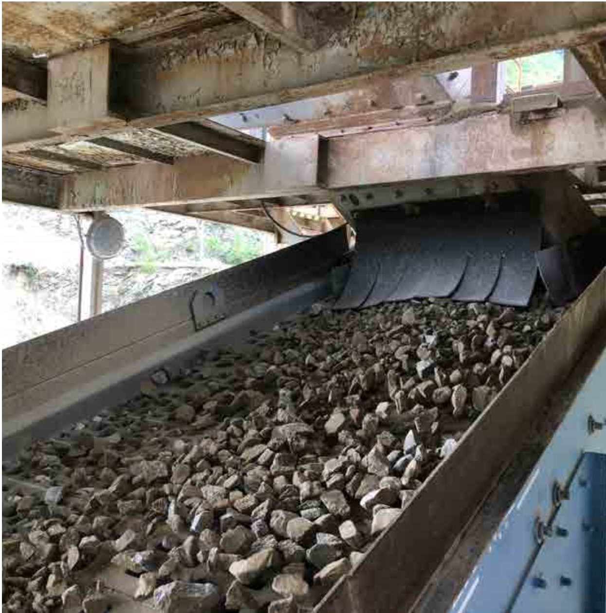
The above image shows an uneven material distribution on screening media. The material has been fed more towards the left hand side of the screen (seen from the top of the screen). The feed bed is thinner towards the right hand side of the screen. An even material flow is to be preferred to ensure your equipment and component's lifespan.
