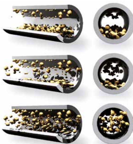
Figure 3: Different flow conditions. The lowest variant represents the preferred flow conditions.
