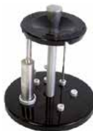
Image 1: Rotational viscometer and spindle set:
