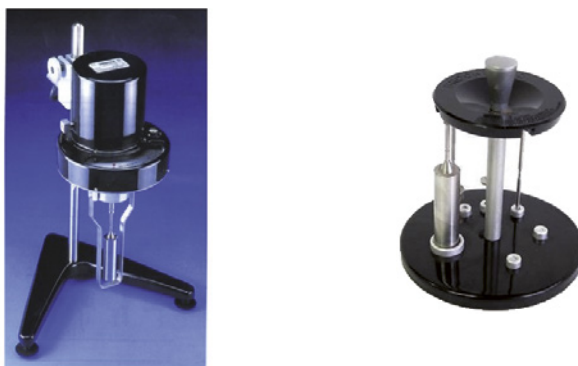
Image 1: Rotational viscometer and spindle set: Courtesy of Brookfield Engineering Laboratories Inc
