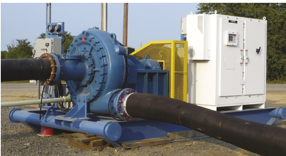
Land based booster dredge pump
