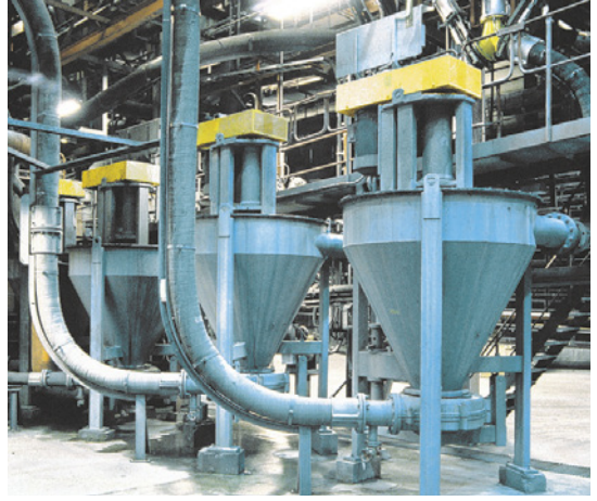
VF pump with vertically mounted motor (shaft up) and v-belt drive.
