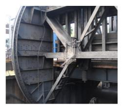
Rolled T end rings Traditional end rings are welded under the end ring rail and subject to high wheel loads. This critical weld often cracks prematurely, leading to end ring failure.
