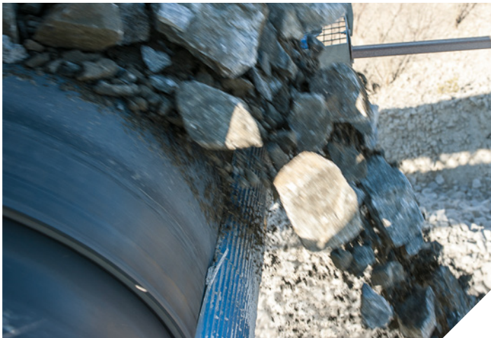
In the majority of cases, the primary belt cleaner is positioned on the head pulley, which is where the material leaves the belt.
