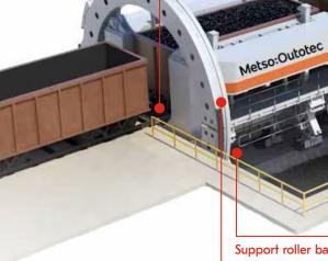
Check the end ring for flat spots, distortion, spalling or damage If present, this will likely lead to your trunnions getting damaged Support roller base grouting is in good condition if present, i.e. no cracks or evidence of the baseplate moving Support roller wear check running and thrust surfaces for excessive wear, pitting or spalling
