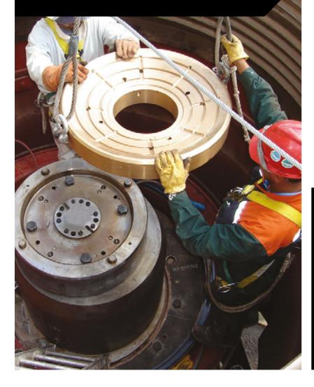
Metso Outotec provides not only the parts for crushers. Our experts can carry out the replacement of major crusher components.
