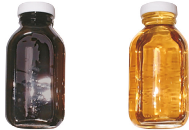
Dirty and clean oil samples, before and after oil filtration. The filter inserts have absorbed the contamination from the crusher oil, and an oil change has now been avoided.
