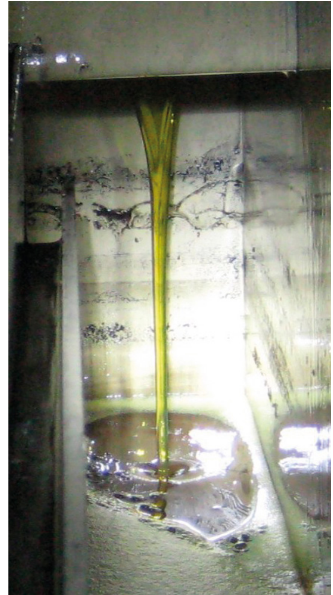
Clean oil is returned to the crusher tank after oil filtration.
