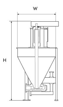
Broad spectrum with the smallest VF pump weighing 355kg and 1.6m tall, while the largest is 5555kg and stands at 4.5m tall
