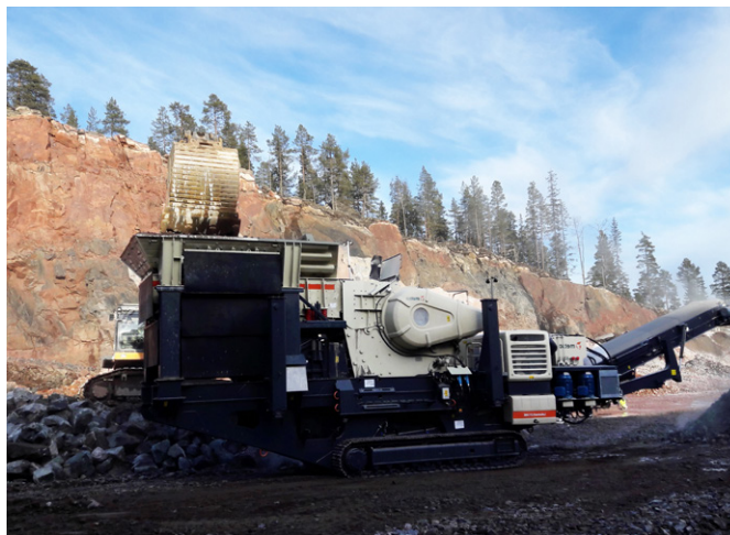
Fully mobile in-pit crushing
