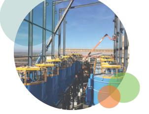
RCS<sup>™</sup> flotation machines are available in sizes 0,8 m<sup>3</sup> to 600 m<sup>3</sup>
