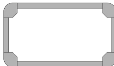
Horizontal closed circuit conveyor (90 degrees) Horizontal routing around a 90-degree bend without transfer.
