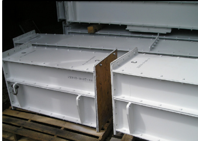
Figure 4: Match-marked casing sections
