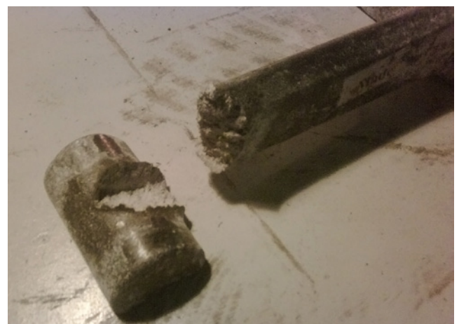
Figure 6: Knuckle broken off from the drawbar of a flight
