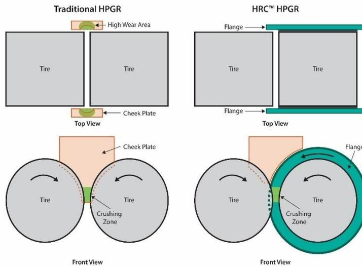
Figure 4 – Comparison of a traditional HPGR with cheek plates versus Metso's HRC™ HPGR with flanges
