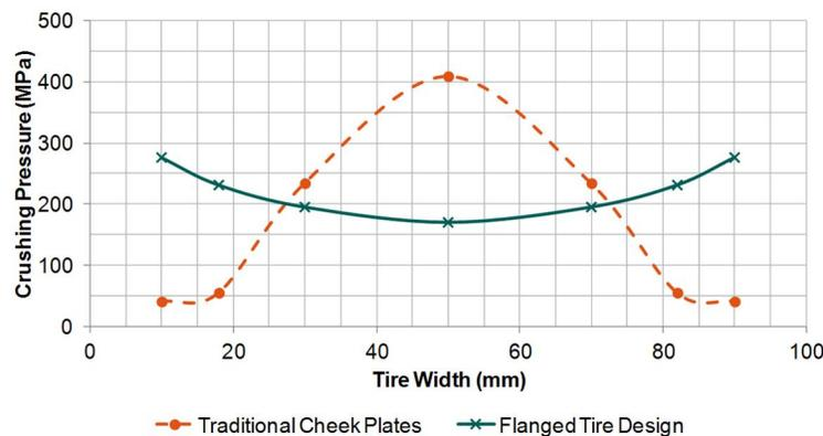
Figure 5 – Pressure profile across width of tire for flanged and non-flanged lab scale
