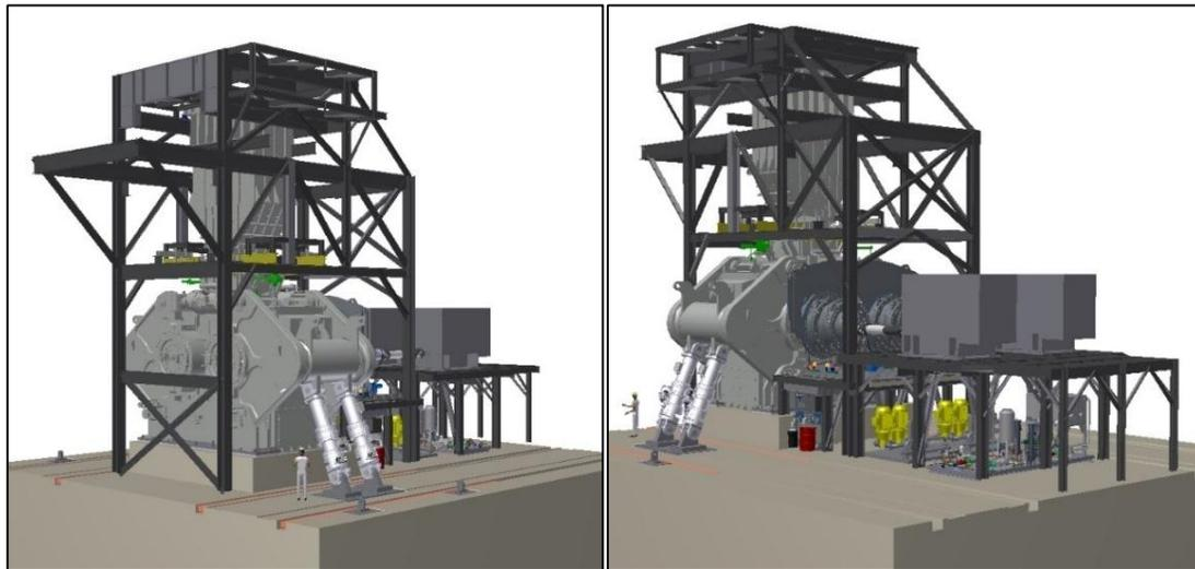
Figure 9 – Steelwork around the HRC™3000
