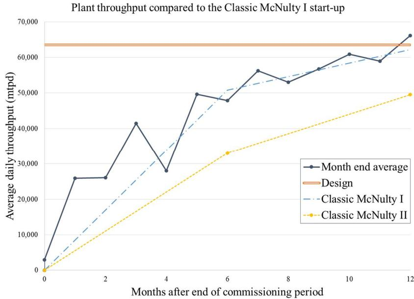
Figure 14 – Metcalf Concentrator daily tonnages versus the Classic McNulty Start-up curve
