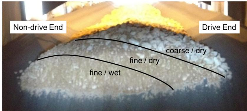
Figure 12 – HRC™ HPGR feed conveyor
