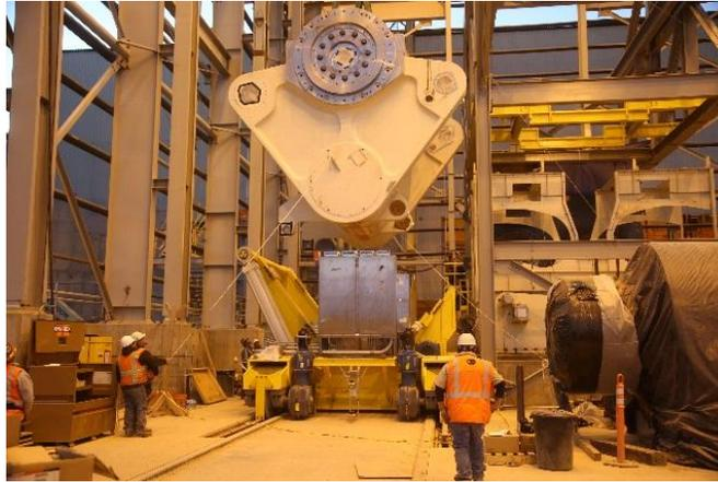
Figure 10 – Morenci transporter for tire removal and installation
