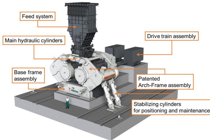
Figure 2 – Main components of HRC™3000
