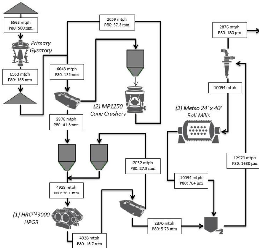
Figure 11 –Metcalfe concentrator design flowsheet
