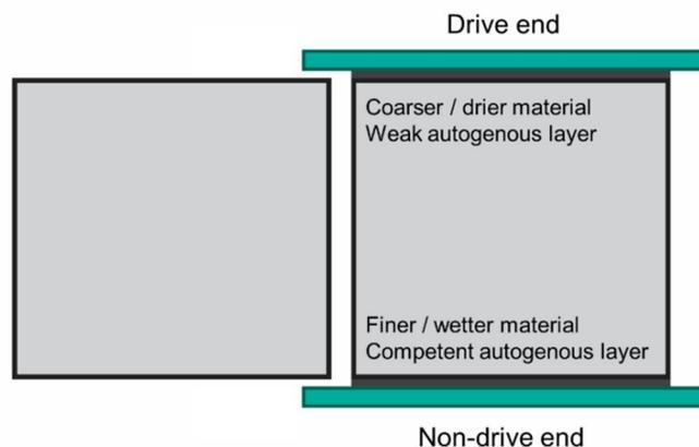
Figure 13 – Diagram of Feed to the HRC™ HPGR
