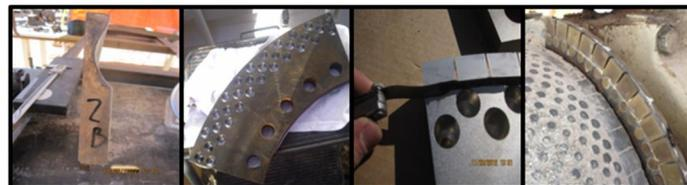
Figure 8 – Progression of flange designs at the pilot plant
