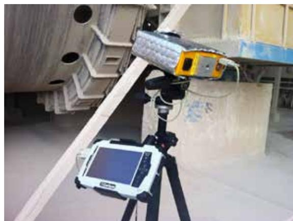
*Unit gathers shell runout measurements and is recorded on field tablet.*
