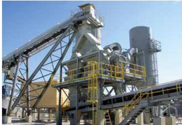
Air classification is a vital aspect in the production of manufactured sand. Two **AC27** gravitational inertial classifiers and one **AC18-9C** classifier in a parallel/series configuration.
