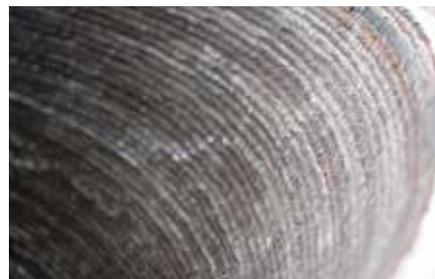
The most classical overlay has the properties of the high chromium iron, but there is also more sophisticated overlays available as well. The clear advantage of the overlays is
