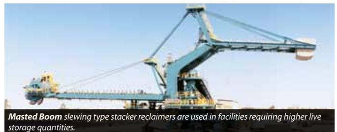
**Masted Boom** slewing type stacker reclaimers are used in facilities requiring higher live storage quantities.
