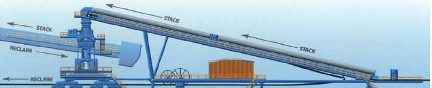
**Articulating Tripper** is used when material enters and leaves the storage area from the same end of the yard. By articulating the tripper structure, this section can be lowered (retracted) for reclaiming operation.
