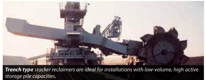
**Trench type** stacker reclaimers are ideal for installations with low-volume, high active storage pile capacities.
