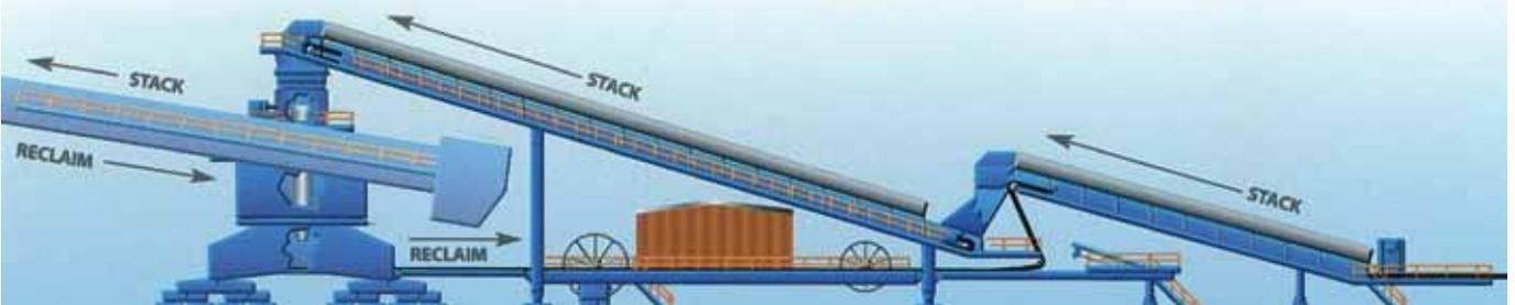
**Scissors-Type Tripper** is also used when material enters and leaves the storage area from the same end of the yard. This tripper utilizes a separate elevating conveyor to direct the material to the centerline of rotation for stacking.
