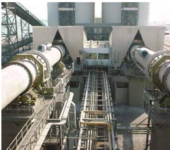
*Two 250,000 MPTY Rotary kiln coke calciners*
