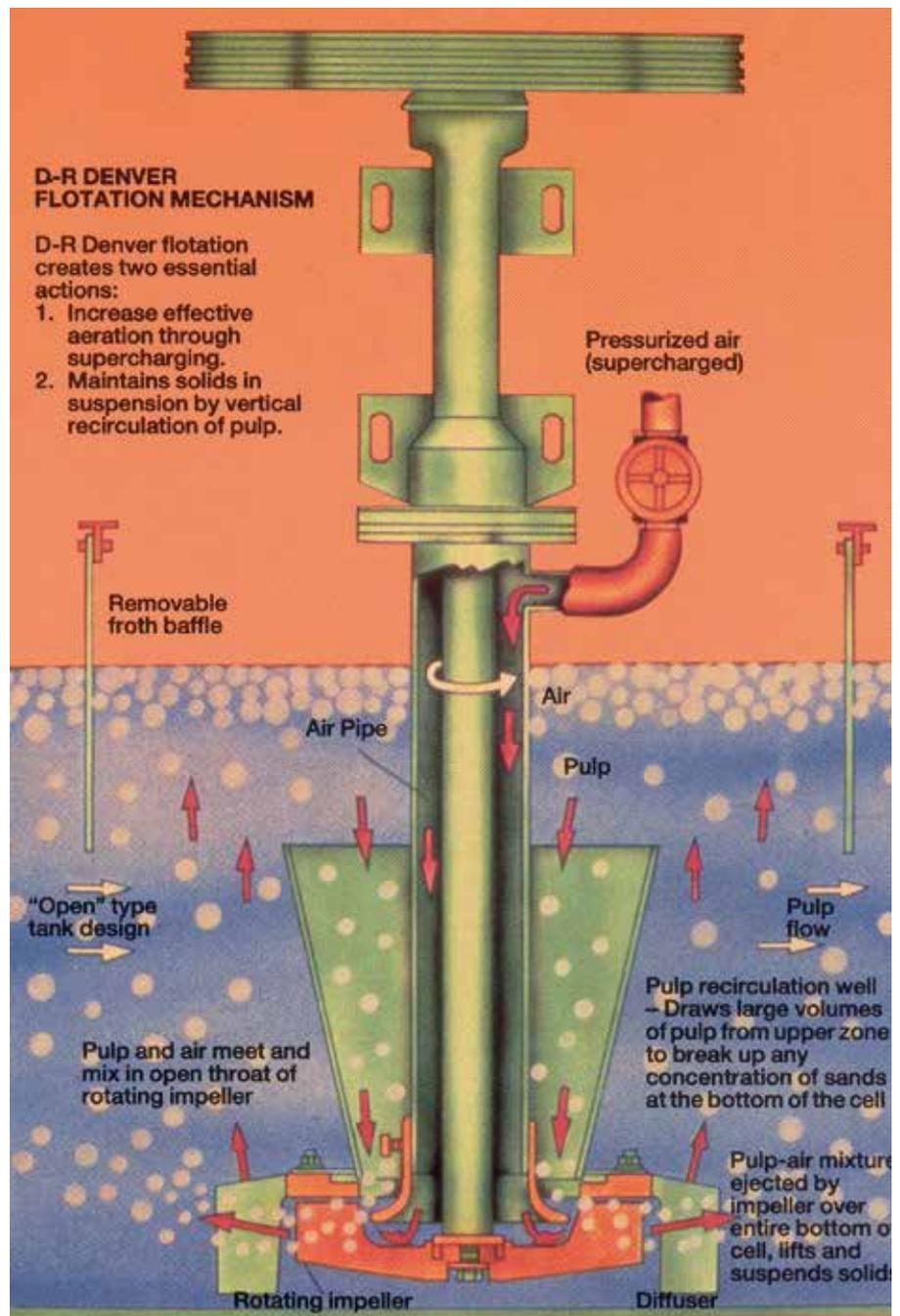
the impeller into the cell creating a homogeneous mixture in the tank. The action is possible only in flotation machines with "top feed" impellers such as used on Metsos DR flotation machines.
