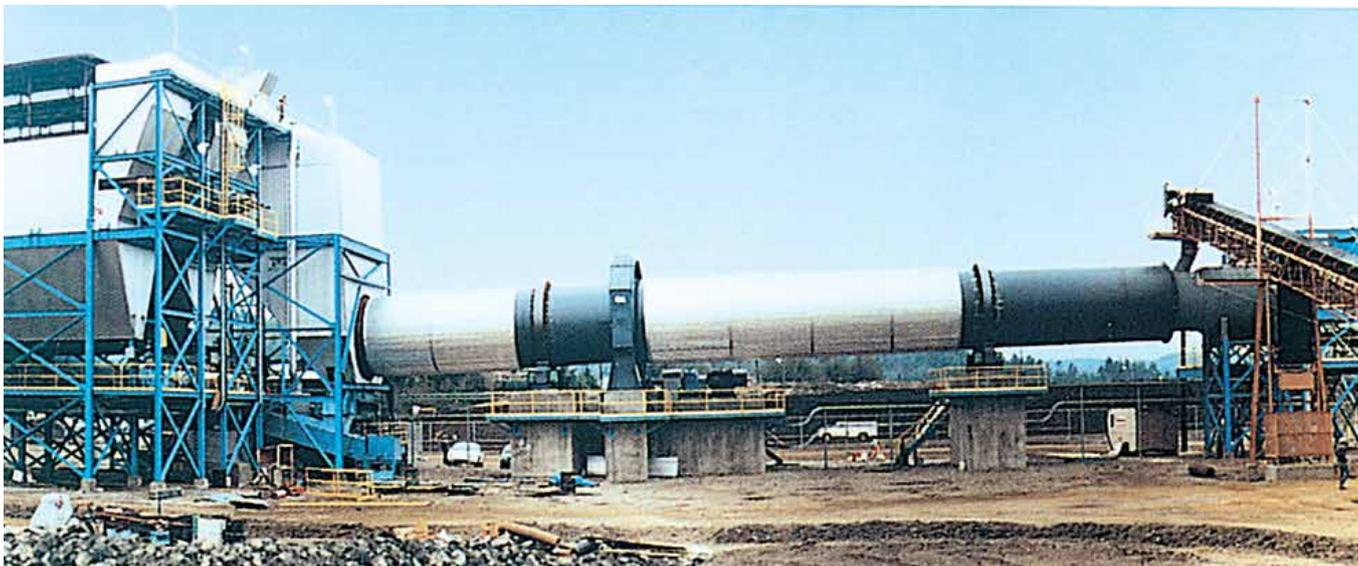
*Nickel ore rotary dryer*
