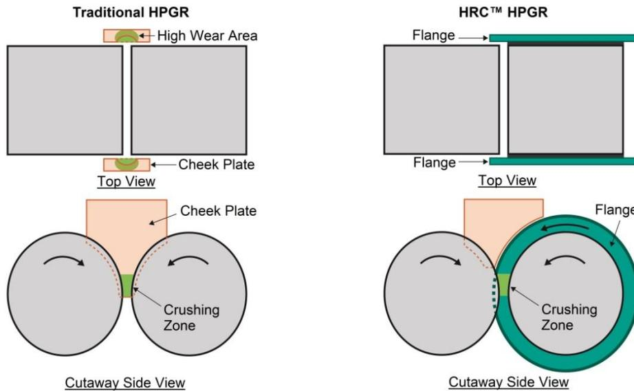
**Figure 1.** Traditional HPGR arrangement (left), HRC™ HPGR arrangement with flanges (right)
