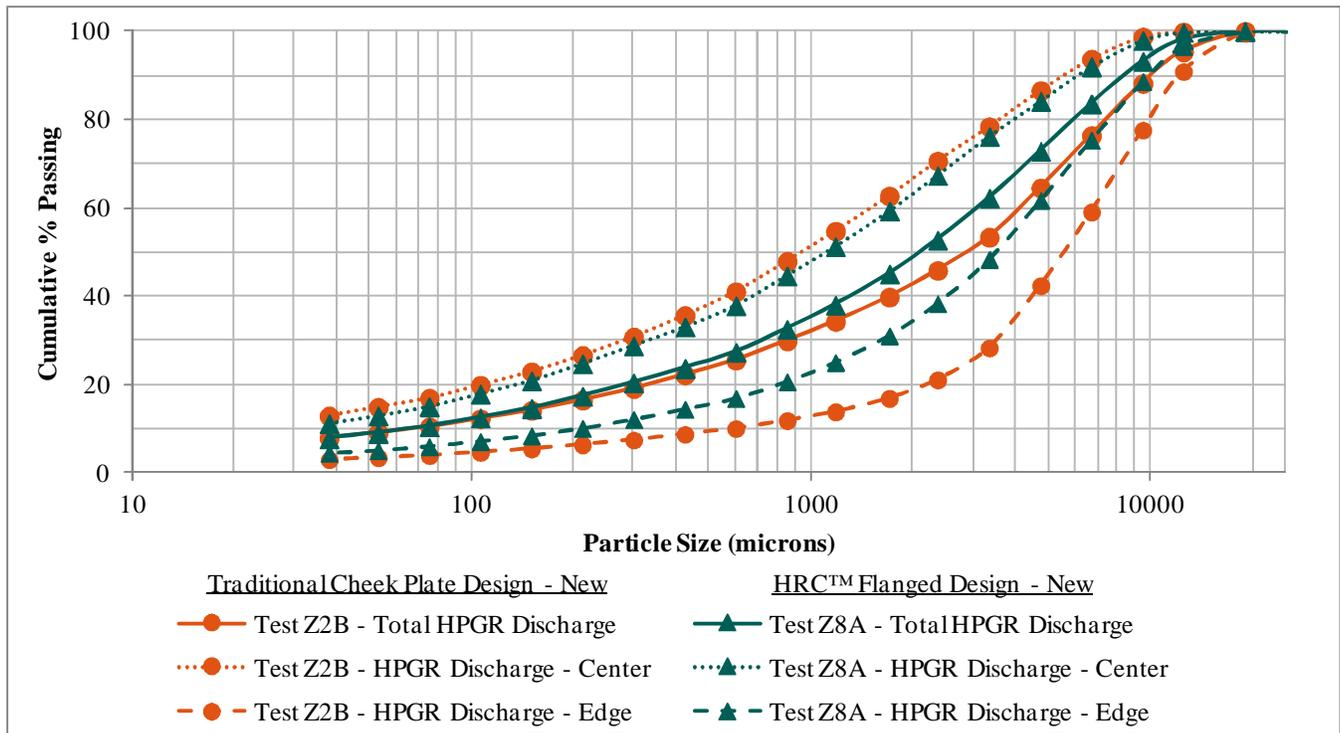
**Figure 3.** Comparison of HPGR discharge samples (total, center, & edge) from tests Z2B and Z8A
