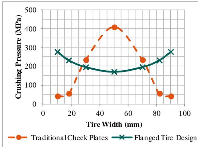
**Figure 2.** Pressure distribution across width of HPGR tire (cheek plates versus flanges)
