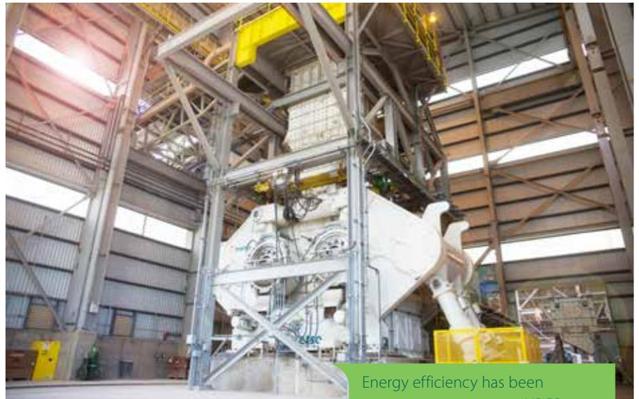
Energy efficiency has been attracting customers to HPGR technology for years. Our new features, the anti-skewing Arch-frame – and the flanges in particular – are increasing machine capacity and further building on the efficiency of the process. That's what is driving customers to choose the HRC™ HPGR.
