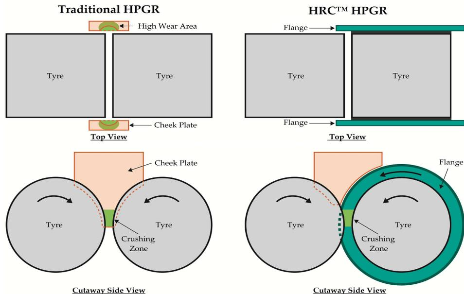
**Figure 1** Traditional HPGR arrangement (left), HRC™ HPGR arrangement with flanges (right)
