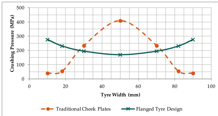
**Figure 2** Pressure distribution across width of HPGR tyre (cheek plates versus flanges)
