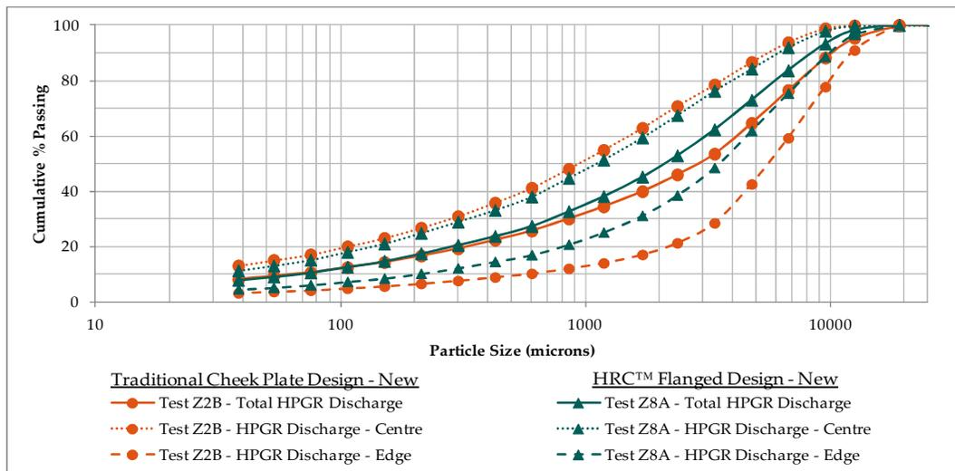
Figure 3 Comparison of HPGR discharge samples (total, center, & edge) from tests Z2B and Z8A
