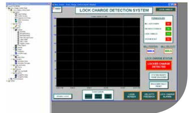
Locked charge detection system screen
