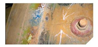
1. Mill Visuals and Vitals: An external crack discovered on a mill shell while performing a visual inspection.
