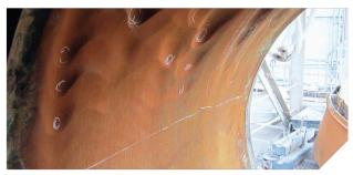
2. Mill Mechanical Verification: Wash pockets discovered inside the mill trunnions. These can be detected from the outside through UT.
