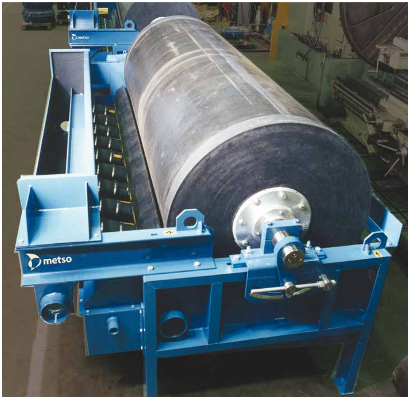
Wet low intensity magnetic separator before shipment to an North American iron ore operation.
