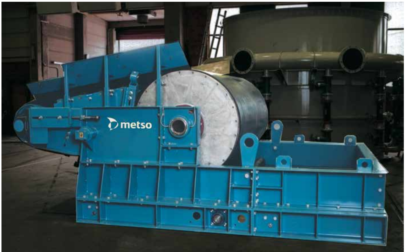
Dry magnetic separator, belt type ready for shipment to an Eastern European iron ore operation.
