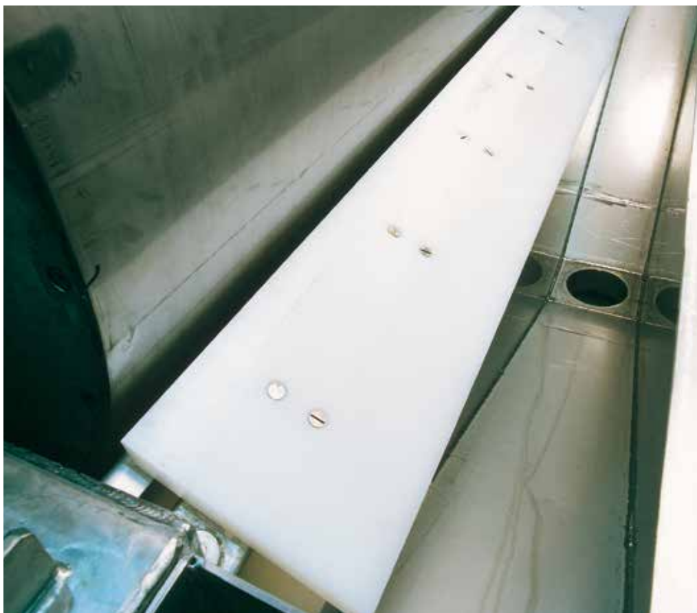
The separator is equipped with adjustable concentrate overflow weir.
