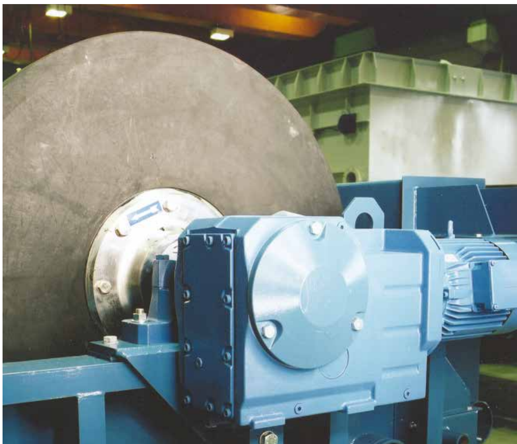
Standard drive system consists of a right angle gear motor
