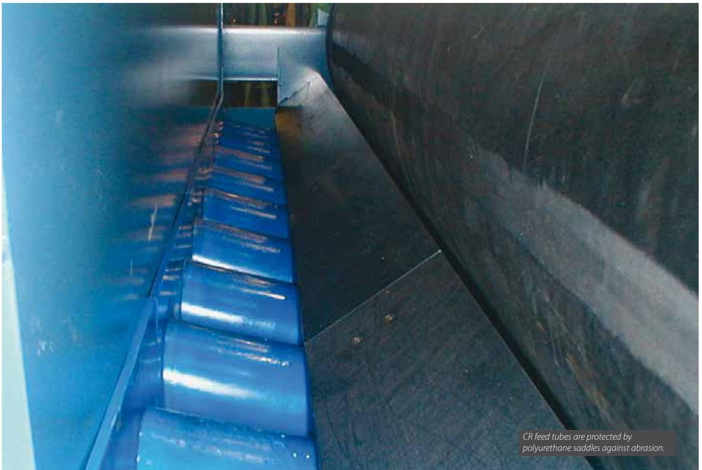
*CR feed tubes are protected by polyurethane saddles against abrasion.*
