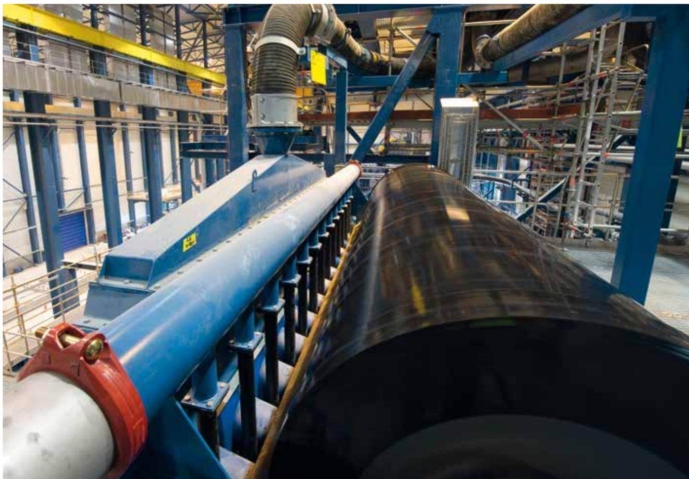
e.g. glass sand and feldspar production. It is also commonly installed for removal of ferromagnetic matter ahead of WHIMS (Wet high intensity magnetic separators) or HGMS (High gradient magnetic separators) units. In dense media circuits LIMS is standard equipment; ask for our special brochure for dense media recovery.
