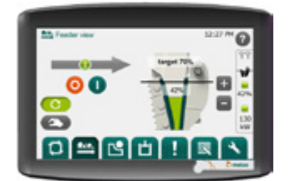
IC10C crusher automation for crushing process optimization and monitoring.
