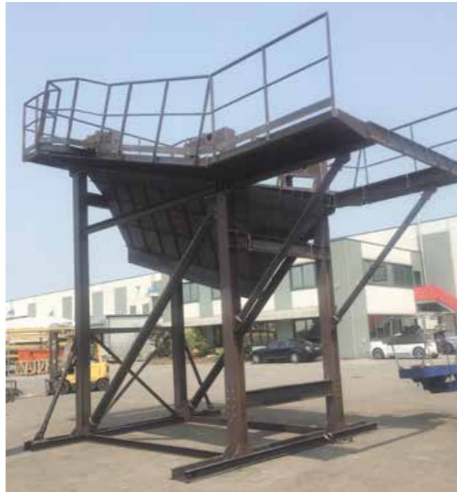
Pre-assembling part of its structural supply before painting guarantees fast and high quality erection on-site.
