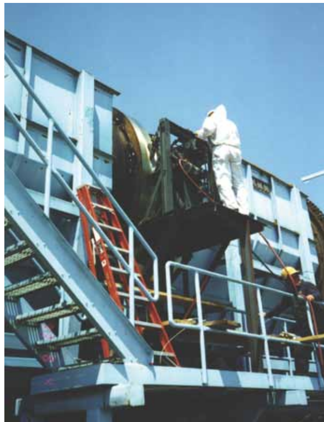
Riding ring resurfacing on debarking drum
