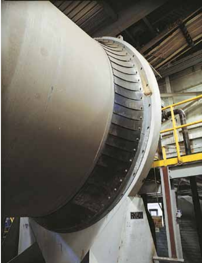
Superdeal seal installed on a kiln for waste recovery.
