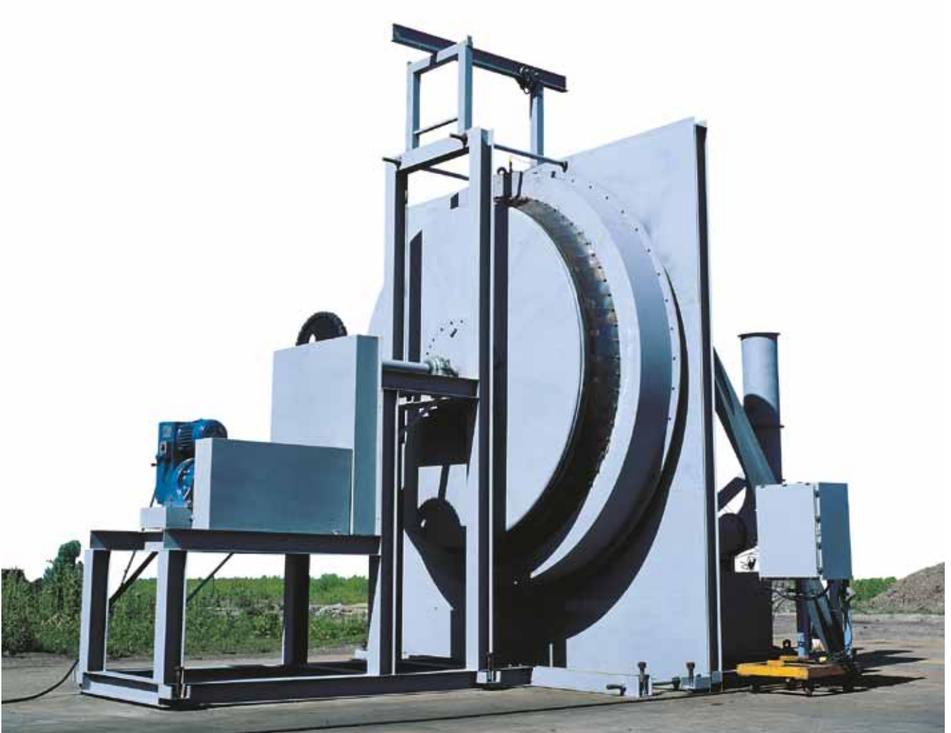
Metso's 10' test unit used for the development and continued improvement in air seal design.
