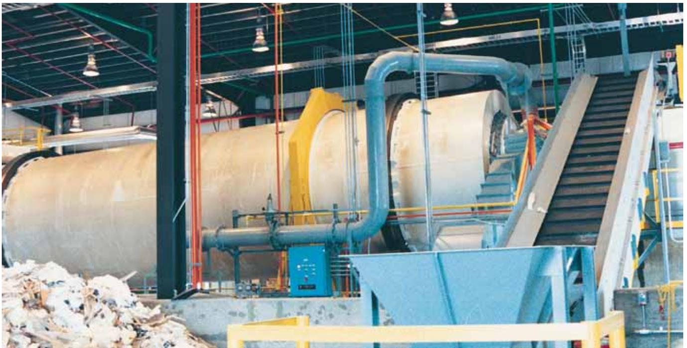
Turnkey, direct-fired 15 X 10<sup>6</sup> KCAL/HR waste incineration system, including boiler and air quality control system.
