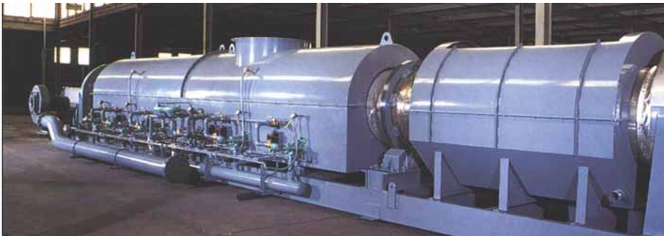
*Integrated indirect-fired rotary kiln and indirect-water film rotary cooler.*
