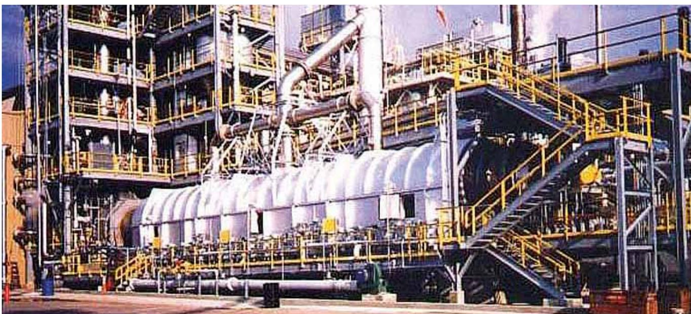
*Indirect heat rotary dryer used for waste processing.*
