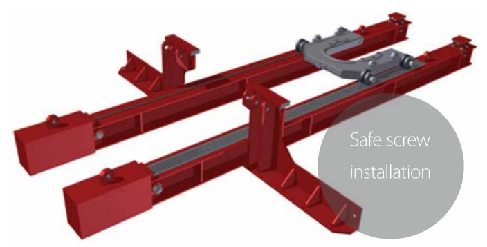
The Vertimill® screw transport system is used for installation and removal of the Vertimill® screw. Two heavy duty beams with a transport cart are included to move the screw into the mill for coupling to the drive shaft.
