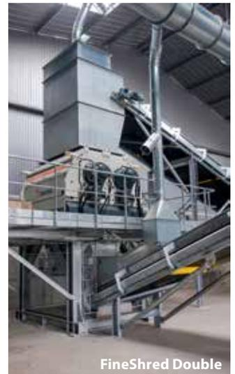
General characteristics for **PreShredders**, available in stationary or mobile models, powered by an electro-hydraulic or diesel-hydraulic power unit, and grain size depends on the number of knives
