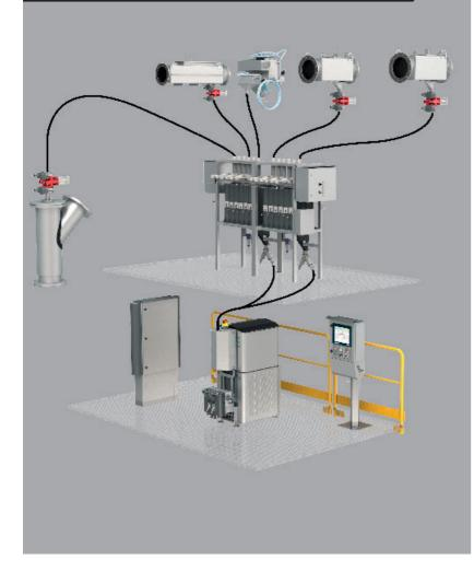
Metso Outotec combines technology innovation and analytics to create the Connected Analytics for Courier. The platform delivers critical event-based equipment conditions and displays operating data of your equipment.
