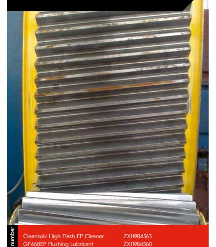
Minimize downtime by removing contamination and lubricant build up on girth gears prior to inspections to get a clear view of the condition of the gear.
