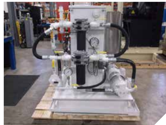
Hydrodynamic lubrication system
