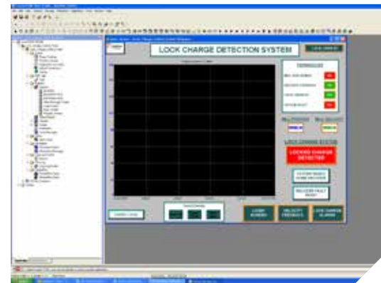
Locked charge detection system screen
