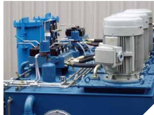
Hydrostatic lubrication system with high pressure pumps
