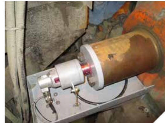
Exposed pinion shaft encoder
