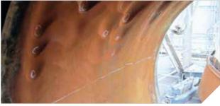
Mill Mechanical Verification: Wash pockets discovered inside the mill trunnions. These can be detected from the outside through UT.
