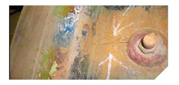
Mill Visuals and Vitals: An external crack discovered on a mill shell while performing a visual inspection.
