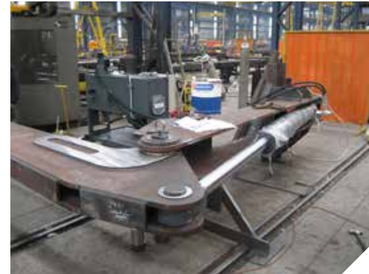
Actuator arm prior to installation
