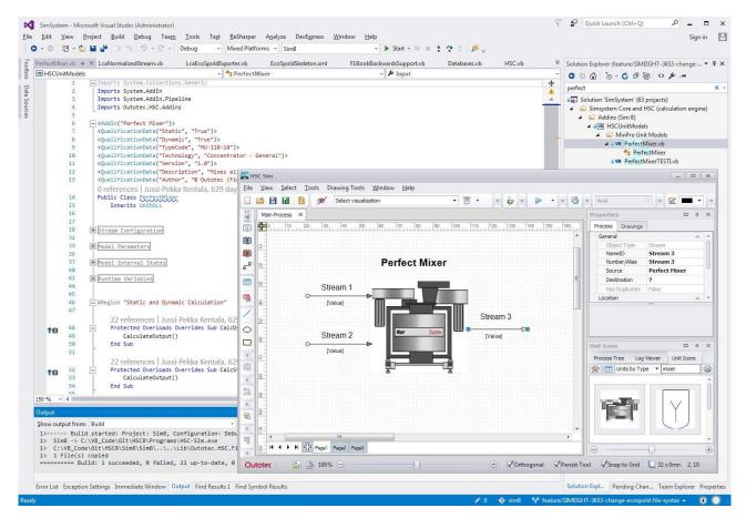
HSC Sim module contains several built-in generic unit operation models of reactors, which users can apply in process flowsheets and calibrate using experimental data. However, users may get full flexibility with their own DLL type unit operation models.
